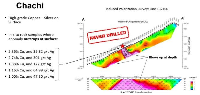
Cross-section of Line 132+00 which crosses directly overtop of a 120m long surface showing of high-grade copper and silver mineralization. Chargeability appears to directly correlate with mineralization on surface.
