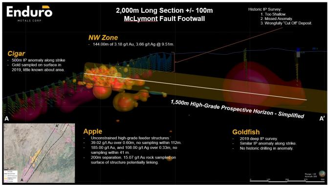
McLymont Fault 2,000m long section highlighting a prospective gold horizon connecting NW Zone and Goldfish. The Apple targets are hypothesized to be narrow, high-grade feeder structures to the NW Zone. Little is known about their potential depth extend, and little is known about Cigar at this time.
