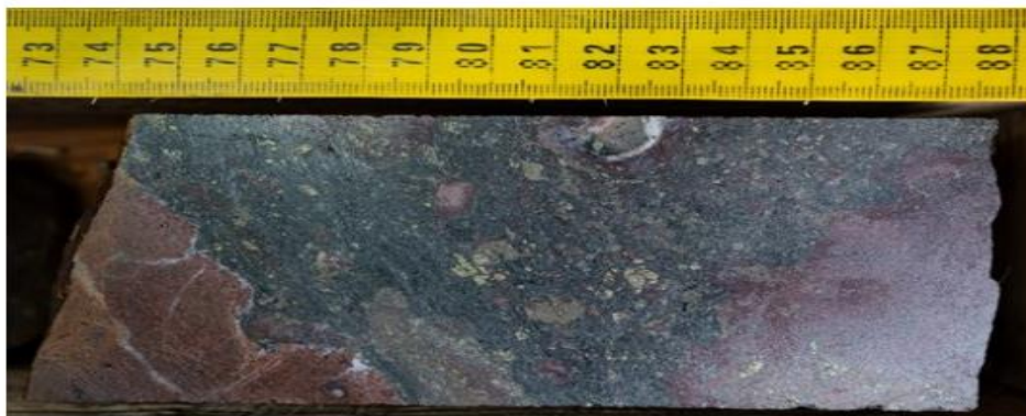
Figure 6: Visual example of "Breccia A" characterized as a heterolithic hydrothermal breccia with a sulphide dominant cement of sphalerite, chalcopyrite, and pyrite. Clasts within the hydrothermal breccia vary in sulphide replacement intensity and phase. It is noted that the larger, more dominant syenitic clasts host what is thought to be "hypogene" chalcopyrite mineralization, indicating that "Breccia A" is a separate mineralizing event which post-dates a "main-stage" mineralizing event. This sample assayed 0.96m of 2.68% Cu, 3.47 g/t Au, 63.26 g/t Ag, and 8.75% Zn starting at 8.53m downhole in BR21-01.
