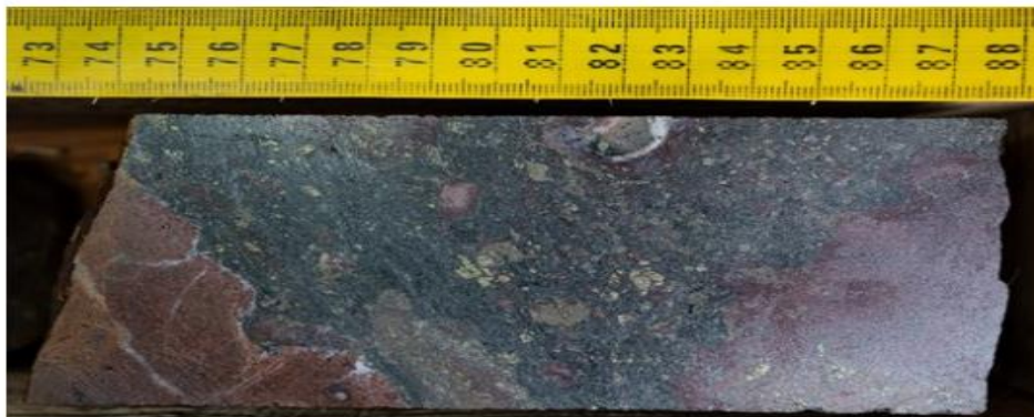
Figure 6: Visual example of "Breccia A" characterized as a heterolithic hydrothermal breccia with a sulphide dominant cement of sphalerite, chalcopyrite, and pyrite. Clasts within the hydrothermal breccia vary in sulphide replacement intensity and phase. It is noted that the larger, more dominant syenitic clasts host what is thought to be "hypogene" chalcopyrite mineralization, indicating that "Breccia A" is a separate mineralizing event which post-dates a "main-stage" mineralizing event. This sample assayed 0.96m of 2.68% Cu, 3.47 g/t Au, 63.26 g/t Ag, and 8.75% Zn starting at 8.53m downhole in BR21-01.
