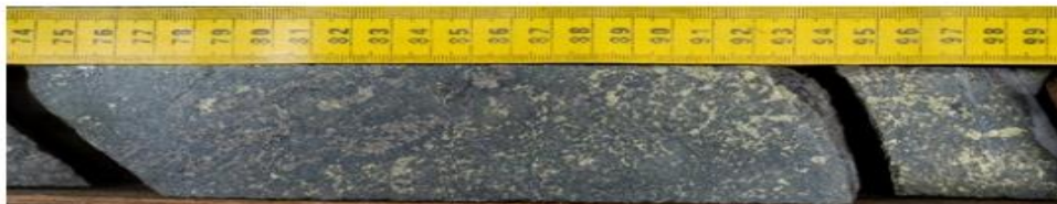
Figure 5: Visual example of "replacement-style" mineralization typical of silica-undersaturated alkalic porphyry systems. Sulphide mineralization is characterized by chalcopyrite, pyrite, and sphalerite. This sample assayed 1.80m of 3.48% Cu, 3.93 g/t Au, 84.73 g/t Ag, and 4.33% Zn starting at 218.6m downhole in BR21-01.
