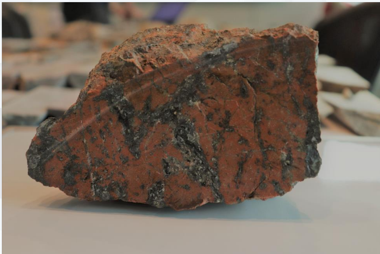
Figure 4: K-feldspar altered rock with chalcopyrite stockwork adjacent to the Green Rock hydrothermal breccia grading 0.46% Cu, 0.53 g/t Au, 10.33 g/t Ag, and 0.32% Zn over 7.00m on surface. Potassic alteration pre-dates the hydrothermal breccia. Zinc content is associated with crosscutting veins of the Green Rock breccia. Winter conditions shut down trench sampling and mineralization remains open.
