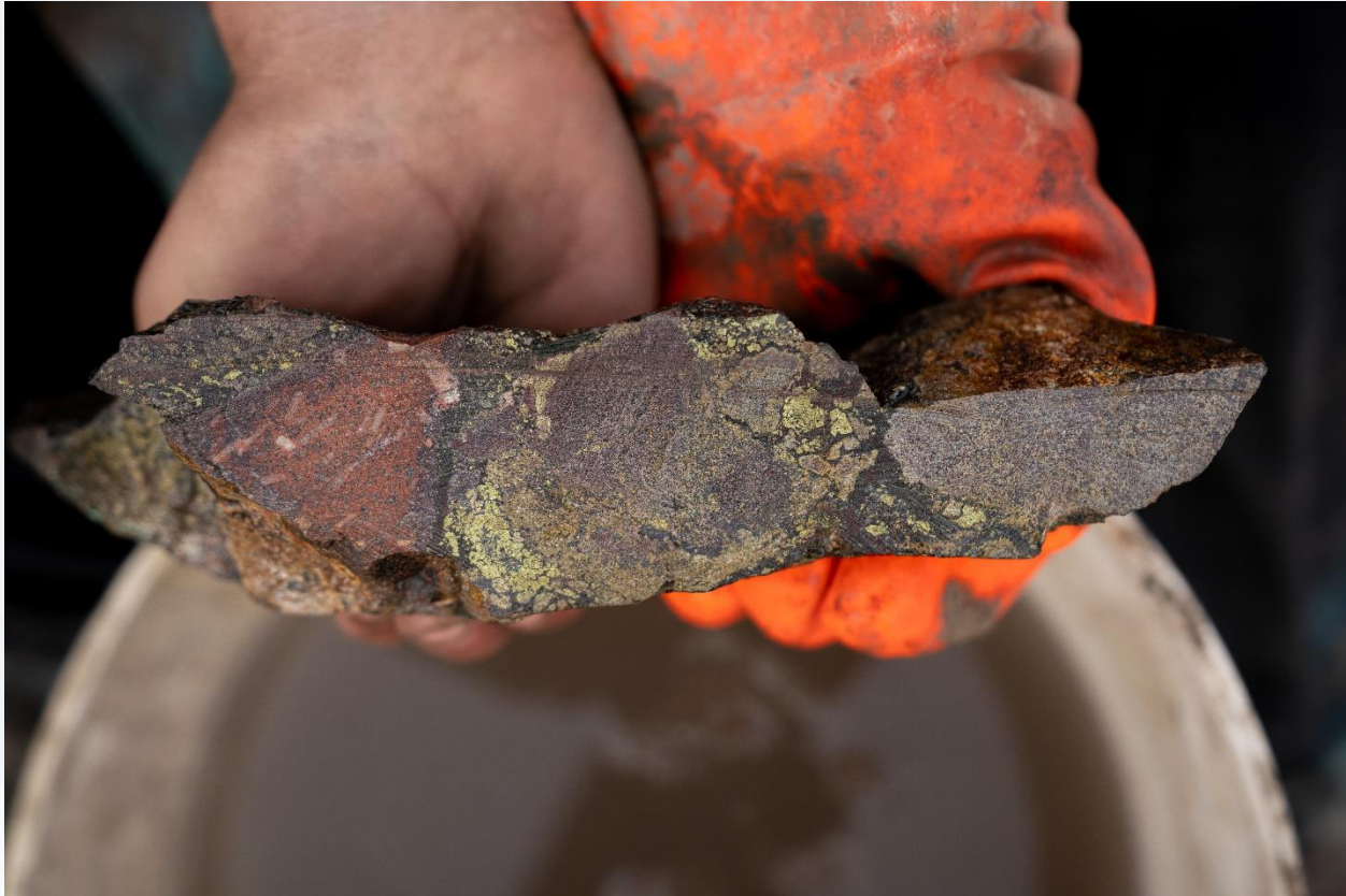
Figure 1: Sample from BRCH19-01 of 3.29% Cu, 8.59% Zn, 3.75 g/t Au, and 63.40 g/t Ag over 10.00 metres on surface. Chalcopyrite, sphalerite, and pyrite cement of hydrothermal breccia is observed. This new showing is ~350m south of drill pad "A-1" at Burgundy Ridge.
